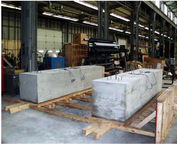
Figure 3.19 Beam Specimens after Formwork Removal
