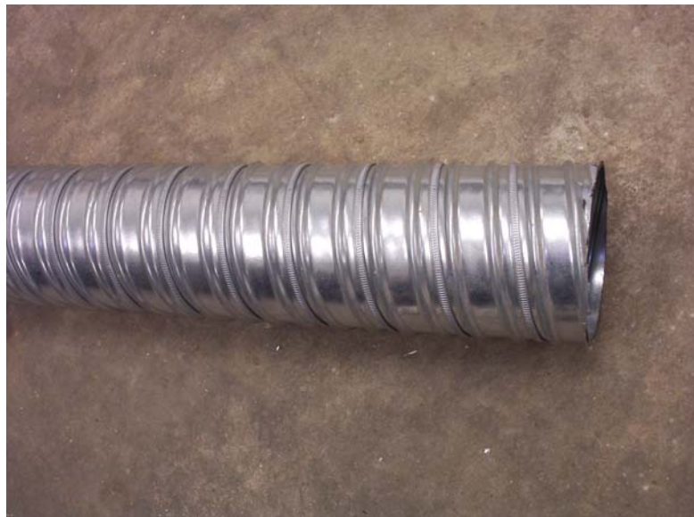
Figure 3.2 Corrugated Galvanized Steel Duct
