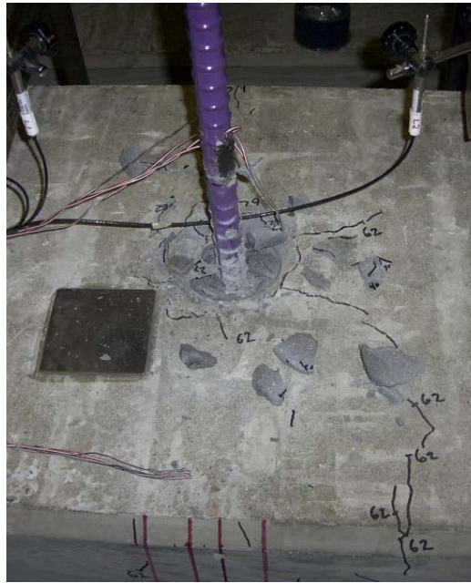
Figure 1.16 Test of Connector Embedded 10d_b [1.14]
