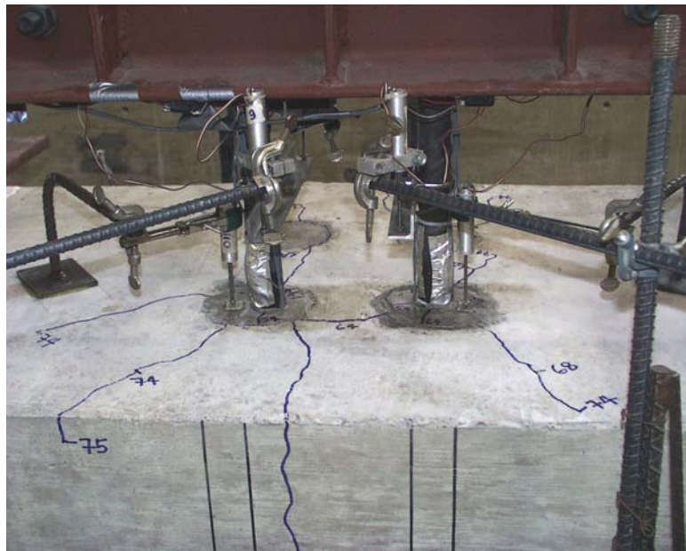
Figure 5.13 Widespread Radial Splitting in Test No. 14
