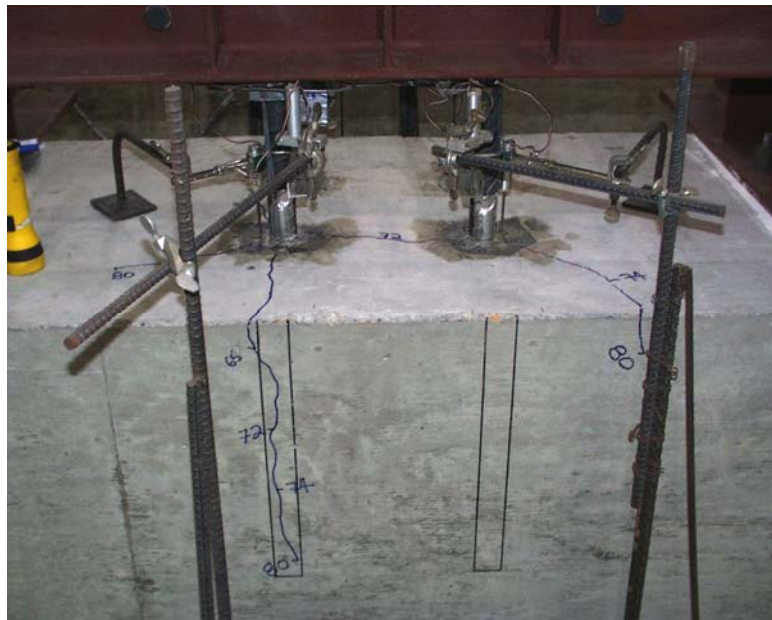
Figure 5.9 Widespread Splitting Cracks in Test No. 23
