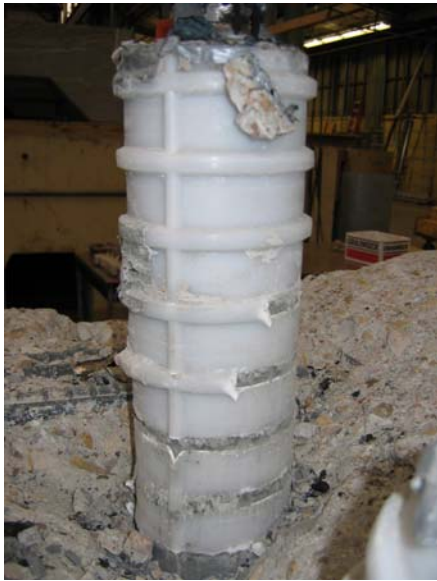
Figure 5.4 Pullout Failure Mode for Polypropylene Duct Connections (Tests No. 30 and No. 32)
