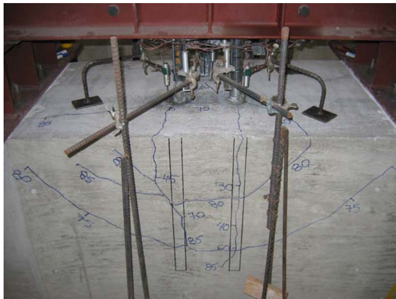
Figure 5.17 V-shaped Crack Formations in Test No. 32
