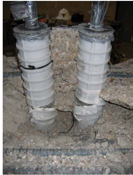
Figure 5.4 Pullout Failure Mode for Polypropylene Duct Connections (Tests No. 30 and No. 32)
