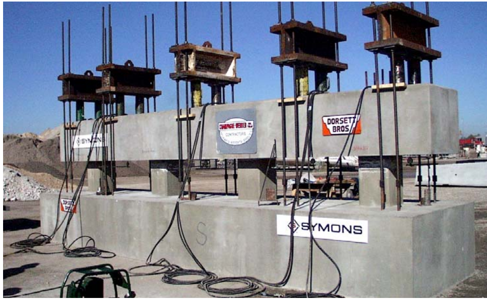
Figure 1.9 Full-Scale Multi-Column Bent of Phase Three (Research Project 1748) [1.5]
