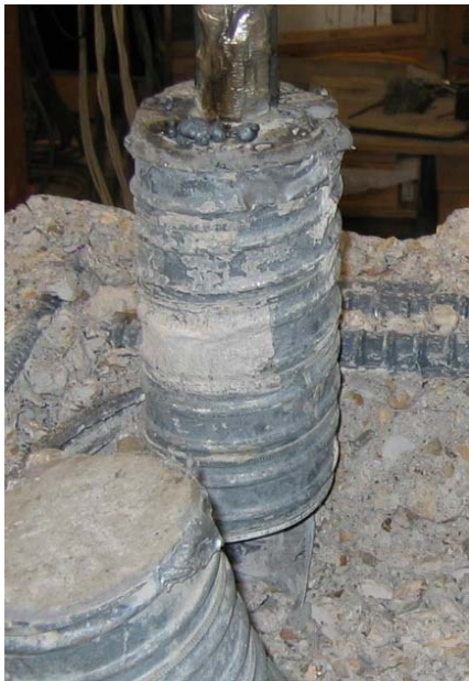
Figure 5.77 Autopsy on Galvanized Steel Duct Specimen (Test No. 23, Left Connector)
