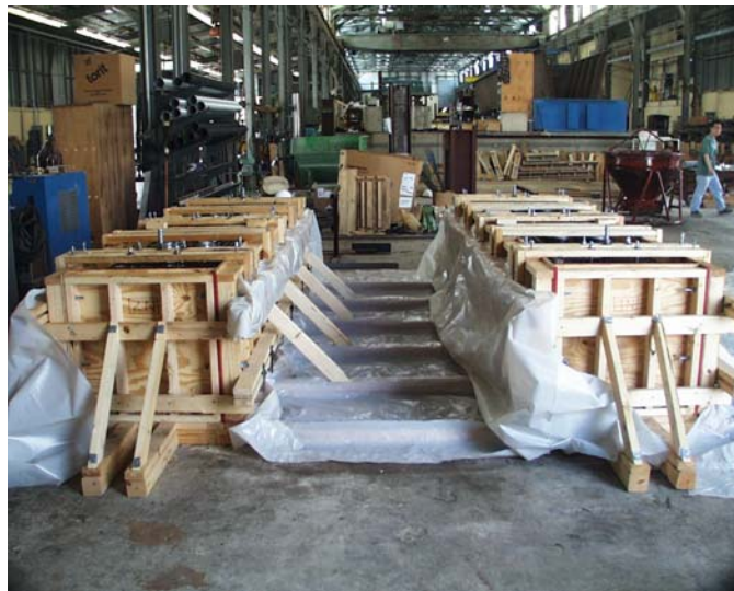
Figure 3.14 Test Specimen Formwork
