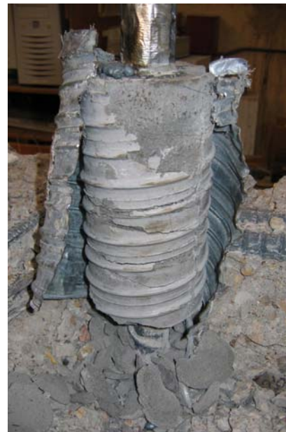
Figure 5.77 Autopsy on Galvanized Steel Duct Specimen (Test No. 23, Left Connector)
