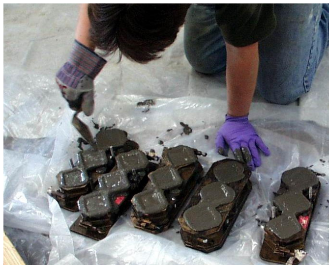
Figure 3.26 Preparation of Grout Cubes
