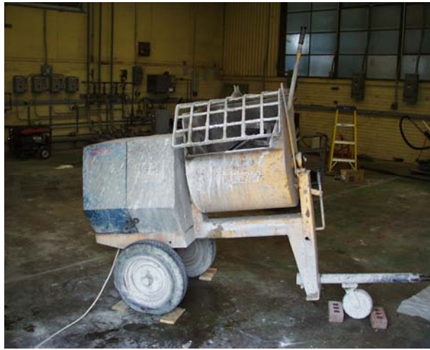
Figure 3.23 Mortar Mixer (2.5 ft 3 capacity) Used to Mix Grout
