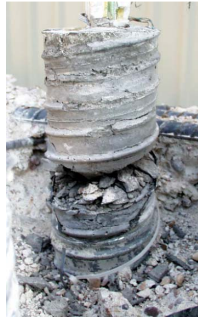
Figure 5.76 Autopsy on Galvanized Steel Duct Specimen (Test No. 4)
