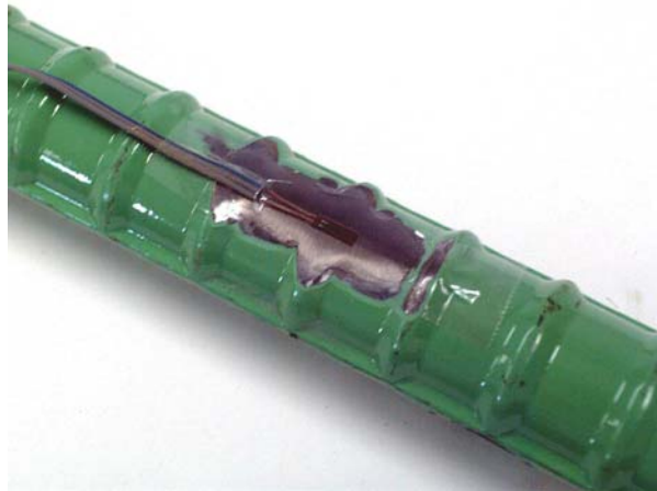
Figure 4.4 Surface Preparations on a Connector for Bonding a Strain Gage
