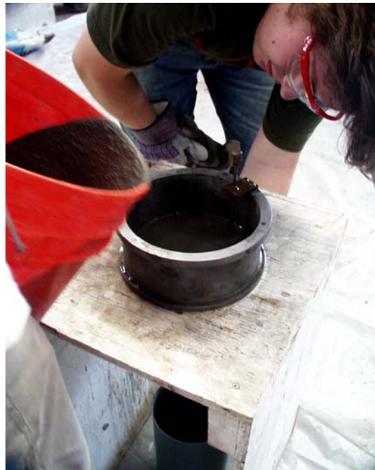
Figure 3.24 Flow Cone Test to Measure the Fluid Consistency of the Grout
