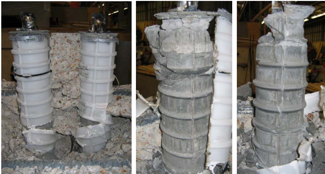
Figure 5.80 Autopsy on Polypropylene Duct Specimen (Test No. 28)
