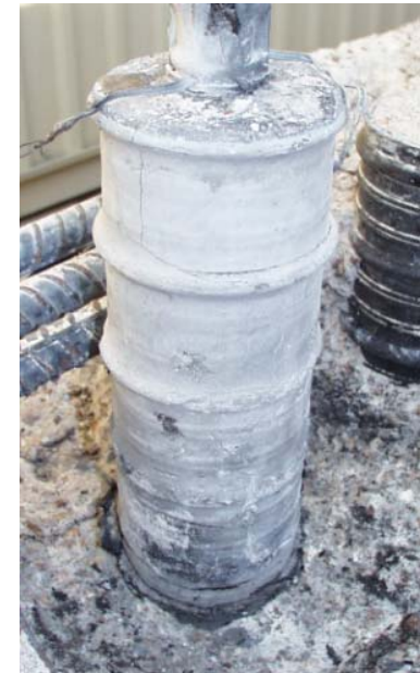
Figure 5.79 Autopsy on Polyethylene Duct Specimen (Test No. 8)
