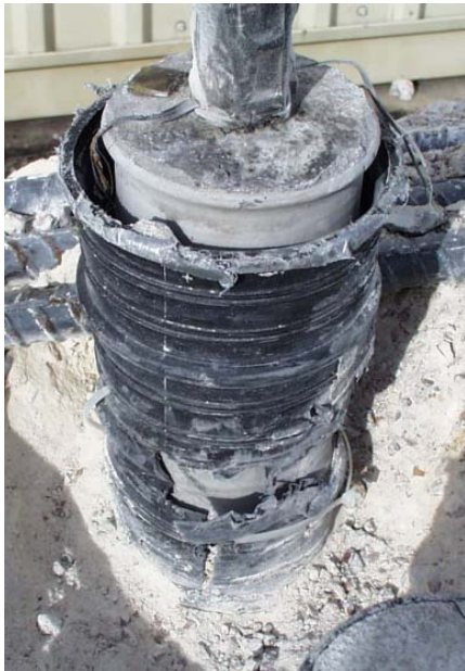
Figure 5.79 Autopsy on Polyethylene Duct Specimen (Test No. 8)
