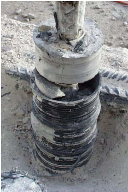
Figure 5.78 Autopsy on Polyethylene Duct Specimen (Test No. 7)
