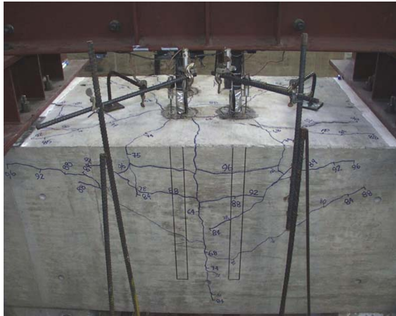
Figure 5.14 Test No. 14 at Failure Load
