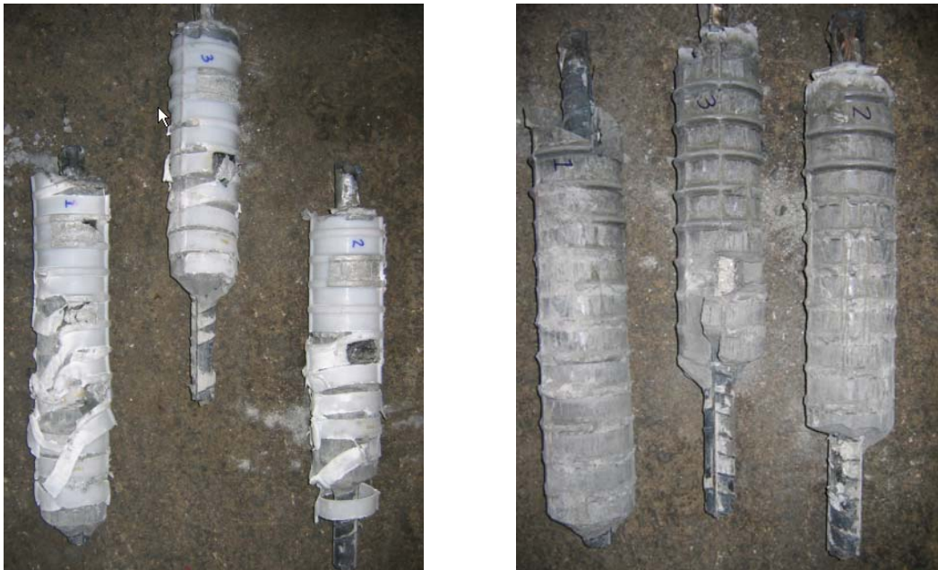
Figure 5.81 Autopsy on Polypropylene Duct Specimen (Test No. 32)
