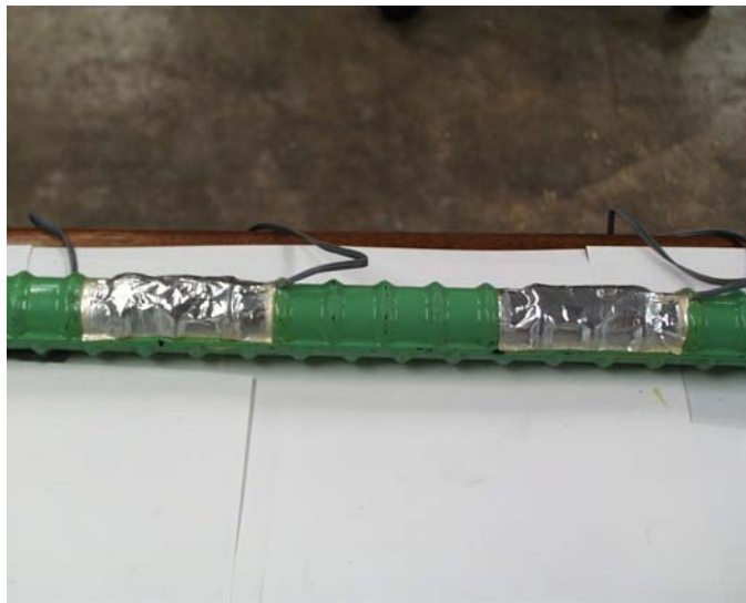
Figure 4.6 Two Completed Strain Gage Installations
