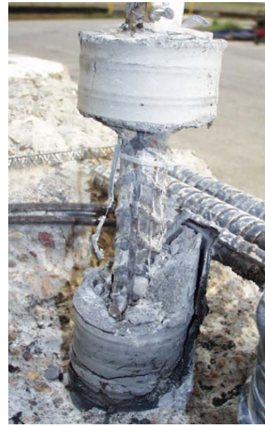
Figure 5.78 Autopsy on Polyethylene Duct Specimen (Test No. 7)
