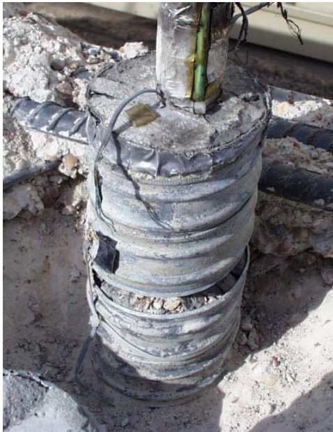
Figure 5.76 Autopsy on Galvanized Steel Duct Specimen (Test No. 4)
